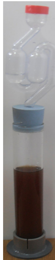
Fig. 1 Fermentation tubes (handmade at Katholieke Universiteit Leuven, Belgium) used to monitor ethanol production through weight loss
